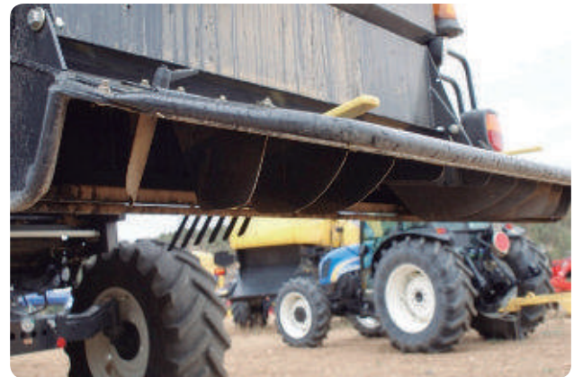
Fig. 3.23. Rear crop residue spreader detail.
