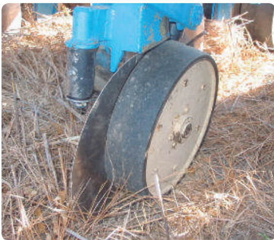
Fig. 3.17. Seeder equipped with single disc opener and lateral depth control wheel.
