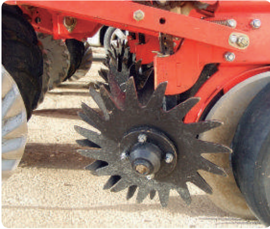
Fig. 3.16. Stubble sweeper mounted on the sowing train.
