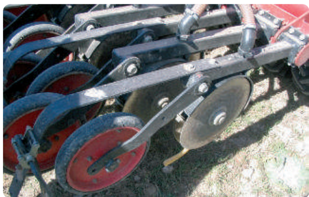
Fig. 3.18. Seed drill equipped with double disc opener.
