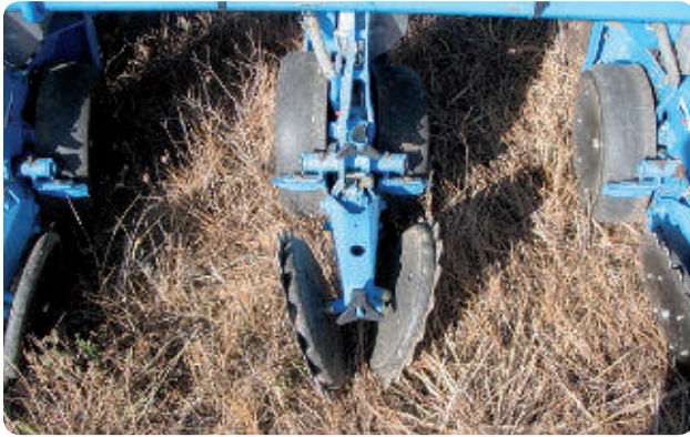
Fig. 3.21. Detail of row closure using double disc.
