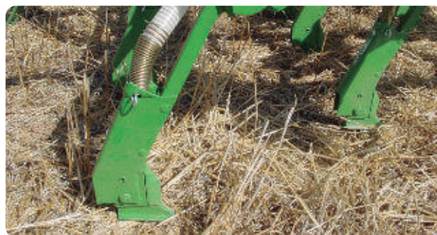
Fig. 3.20. Seed drill equipped with tines.
